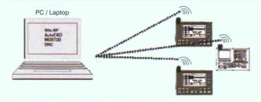
Cub series profile cutting controllers are Bluetooth ready. With such devices, it is possible to connect several CNC's in the plant to a central computer. It is even possible to exchange data between 2 or more CNC's. This state of the art technology reduces cabling costs substantially and can be effectively used for data transfers.
