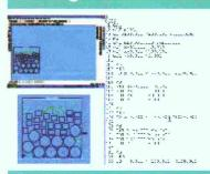
A good nesting software helps the user in achieving precise tolerances of cut parts, high productivity by nesting, less wastage and zero down time. Features include auto Validation, Simulation, Dimension / Enquiry functions, Lead-in Styles, Cutting Parameters, Corner Loops, Offcuts & Scrap Cuts, Grain Alignment, etc
